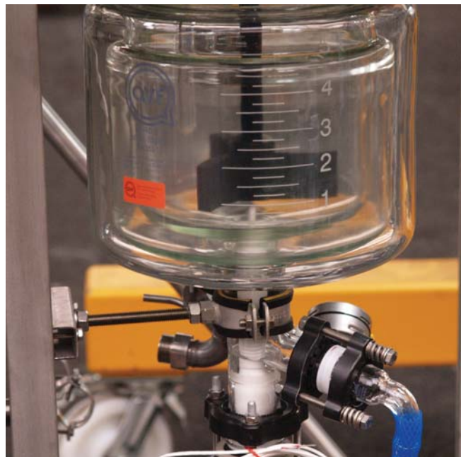
Illustr. 4: Bottom outlet valves employed in triple-wall vessel
